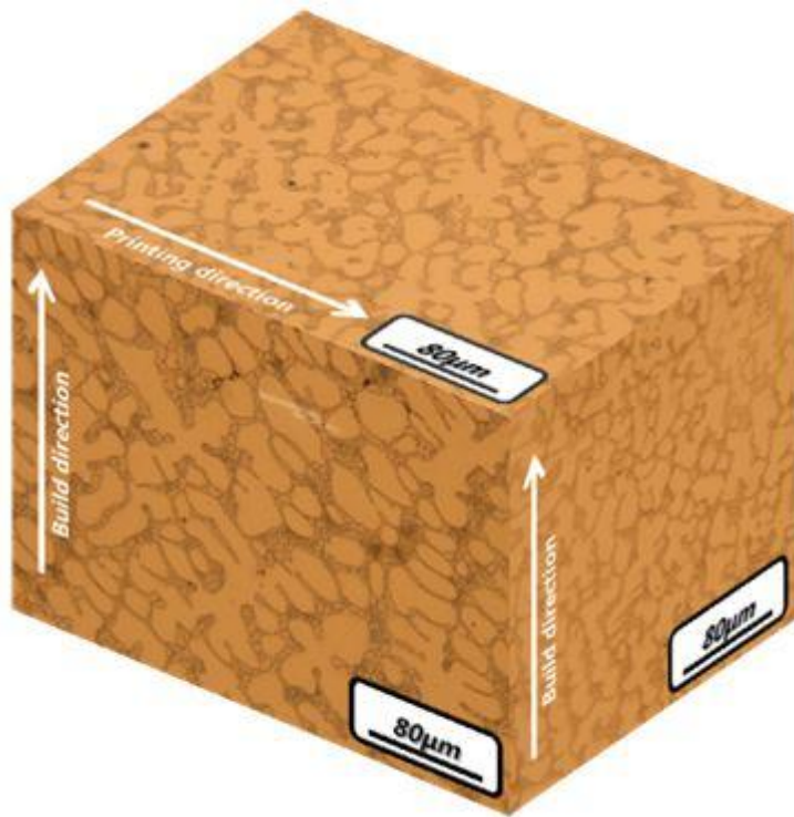
Fig. 1 Initial microstructure of laser metal deposited Ni-1.6%Si.
