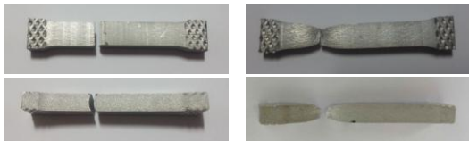
(a) Welding line fracture (b) Ingot-Al fracture
